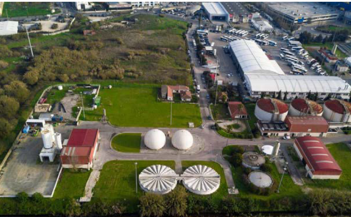
Portugal produces a large proportion of its biogas with sewage gas. This photo shows the Frielas plant, which also processes the biogas into biomethane.
